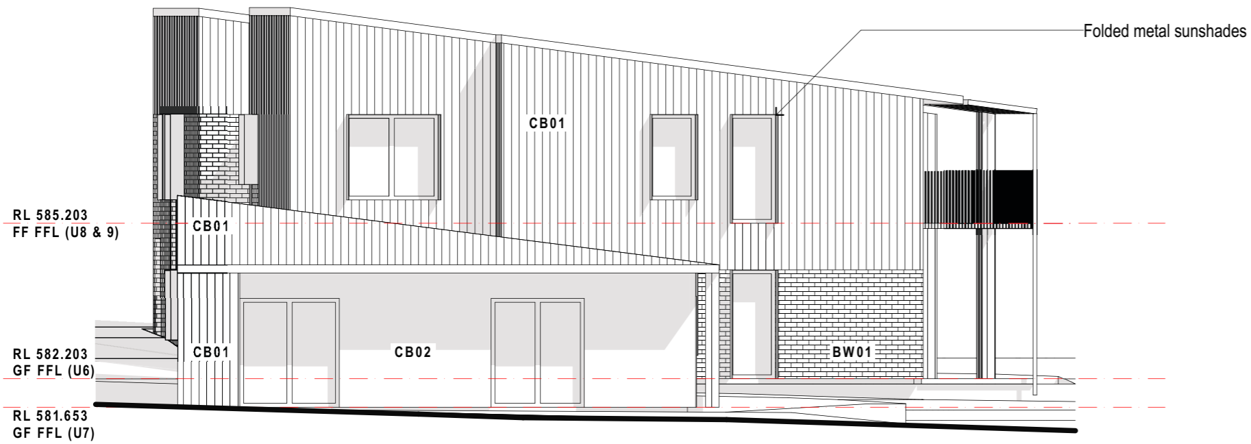
EAST ELEVATION (ACT HOUSING SITE) SCALE 1:100 @ A3
